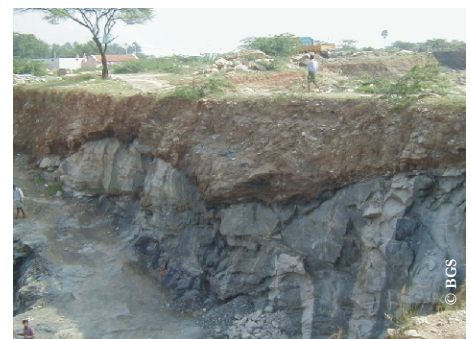
A quarry showing a shallow weathered zone overlying fractured hard rock
