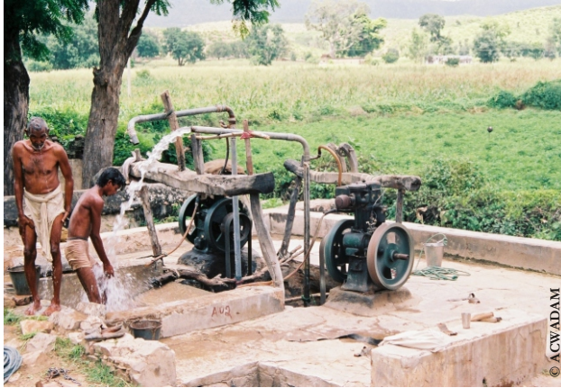
Two diesel engines pumping out water from a dug well in the Arwari basin, Rajasthan
